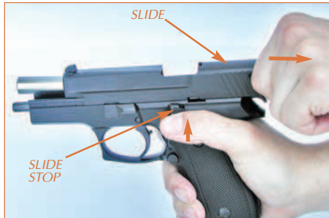
Fig. 9 PULLING SLIDE BACK IN THE REAR POSITION
