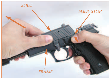
Fig. 11 SEPARATING SLIDE FROM THE FRAME
