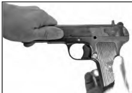
Fig. 8> Separating the slide
