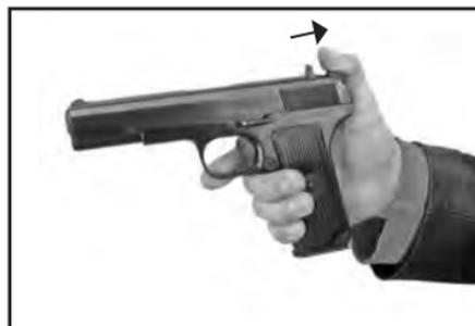
Fig. 4> Blocking the trigger with the hammer lowered
