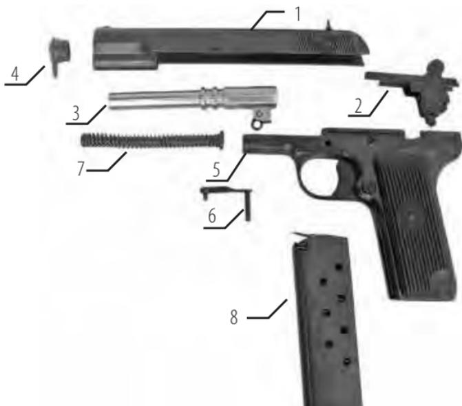
Fig. 13> Stripped pistol
