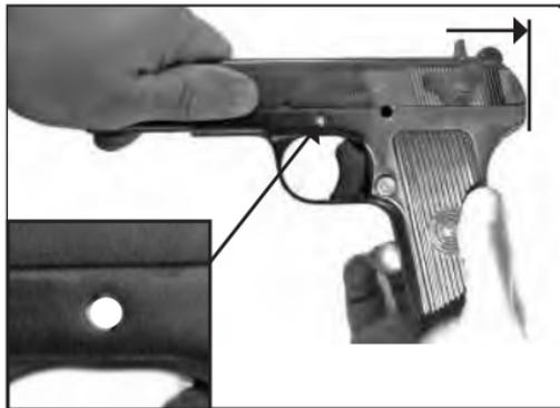
Fig. 15> Position of parts before inserting coupling
