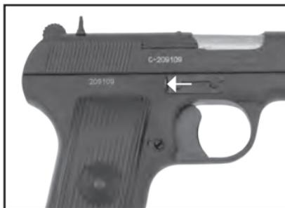
Fig. 6> Separating the coupling
