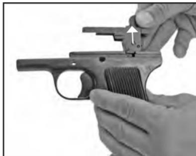
Fig. 9> Separating the trigger mechanism from the frame
