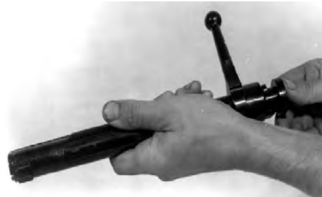
Fig. 16 – Stripping of the bolt
