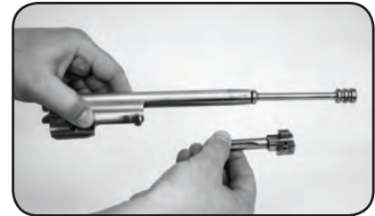
Picture #15 Separate bolt from carrier
