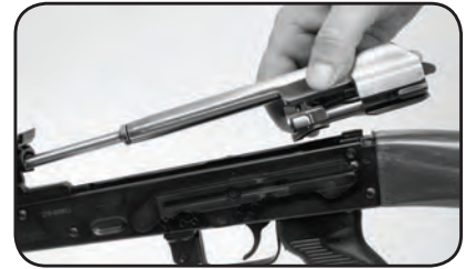
Picture #14 Remove bolt and carrier
