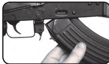
Picture #9.1 Attaching the magazine
