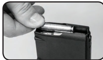
Picture #8 Loading cartridges
