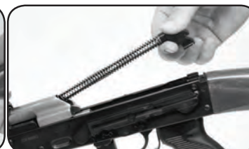
Picture #13 Remove the recoil spring
